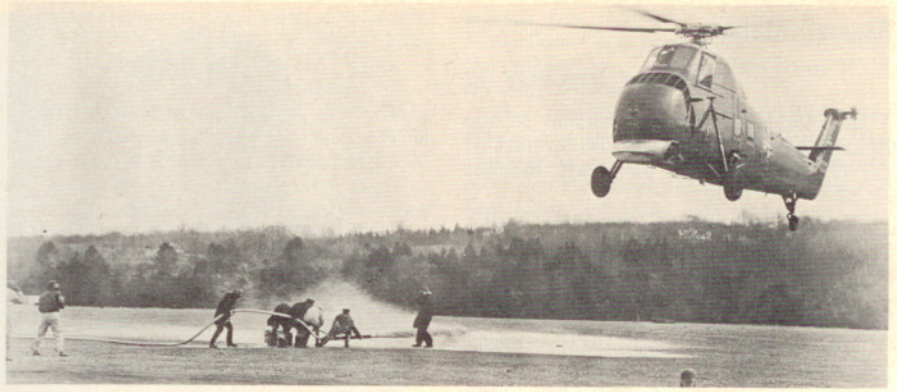
After unloading, helicopter hovers overhead to help extinguish fire by its downwash
